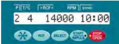
The MIKRO 200 / 200 R, MIKRO 220 / 220 R, UNIVERSAL 320 / 320 R and ROTOFIX 46 / 46 H models are quick and easy to operate using this variant of the N control panel. The parameters are selected with the Select key. An adjuster knob is used to set the values, and the settings are stored by pressing the Start/Impulse key.
